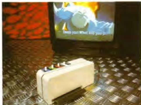
The Video Digitiser 2 plugs into the expansion slot at the side of a 500, and the controls are at the back!
